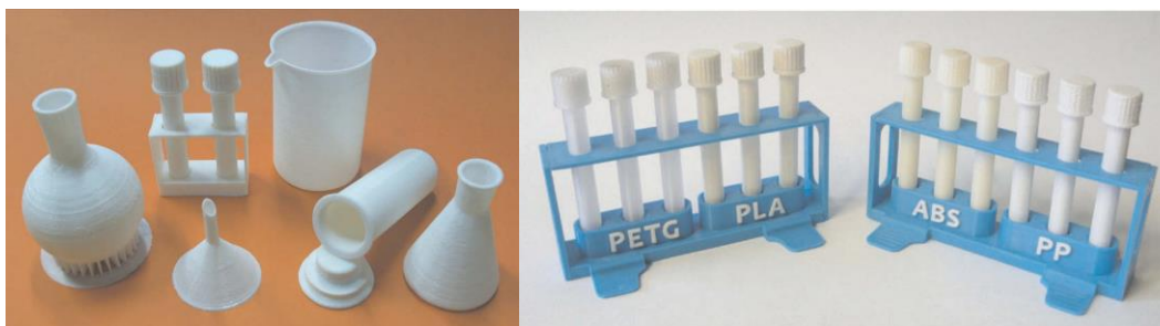
Figure 5. a) Examples of labware typically used in chemistry laboratories printed by an FDM 3D printer b) test tubes produced with different filaments. Reproduced with permission from Ananikov et al. 53
